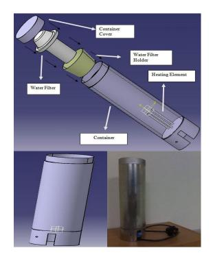
Fig. 3. Portable Water Filter Assembly.
