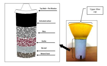
Fig. 2. Filter Cartridge and its Layers.
